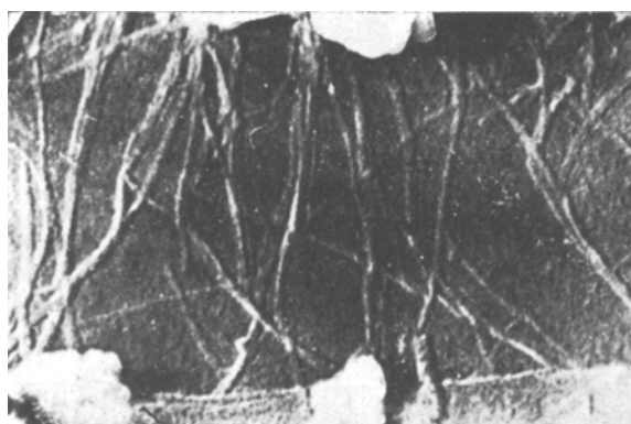
Fig. 3. Electron microscopic photomicrograph of poly[2,5-(p,p'-diphenylenephthalide)]-1,3,4-oxadiazole after subjection to ultrasonic dispersion.
