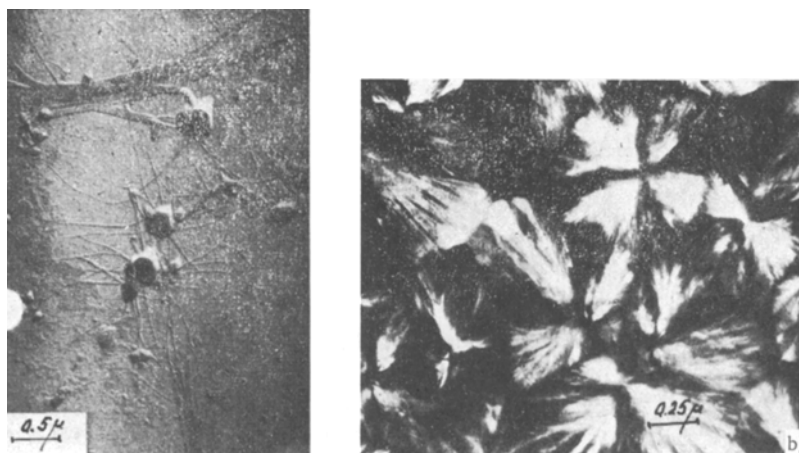
Fig. 2. Electron microscopic photomicrographs of the surfaces of films (100–300 Å) of amorphous (a) and crystalline (b) poly[2,5-(p,p'-diphenyleneoxide)]-1,3,4-oxadiazole.
